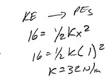
If the cart comes to rest after compressing the spring a distance of 1.0 meter, what is the spring constant of the spring?
